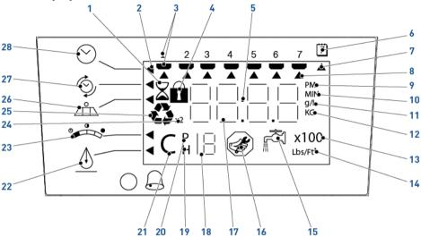
1. Hourglass Displayed when the motor is running. The camshaft should be turning.
